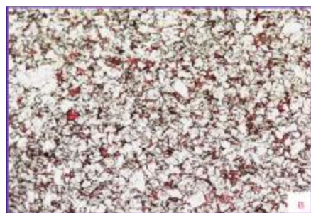
(a) 粉晶白云岩, 白云石晶径达0.05~0.08mm, 半自形镶嵌结构, 含晶间孔10%左右(氮孔隙度9.6%)。单偏光, \times 100 , 铸体片, 陕201井马五 1 2 , 5-78/132, 2865.58~2865.60m
