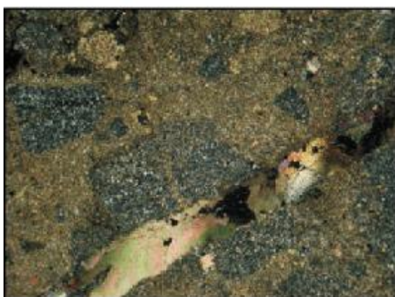
(c) 强碎化构造角砾含白云岩,易鞍状白云石脉切割角砾,上震旦统灯影组,林1井,2647.75m。(+)×4
