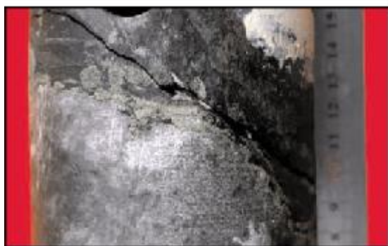
(g) 岩溶角砾岩, 黄铁矿充填于裂缝。A19井3753.16~3753.24m, 岩心
