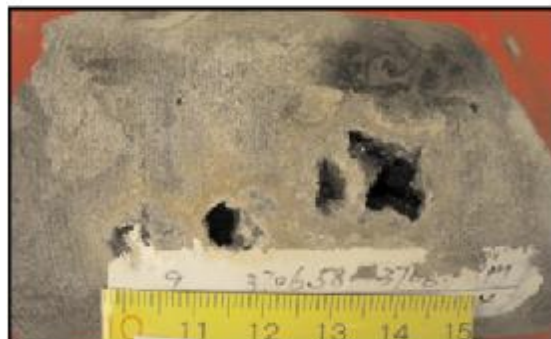
(e) 泥质泥晶白云岩。见溶孔溶洞, 被石英半充填。A172井3706.58~3706.68m, 岩心
