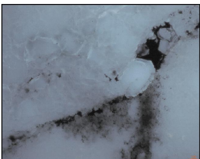
(b) 沥青充填裂缝之中。顺3井6441.47m, 上奥陶统良里塔格组。荧光, \times 20
