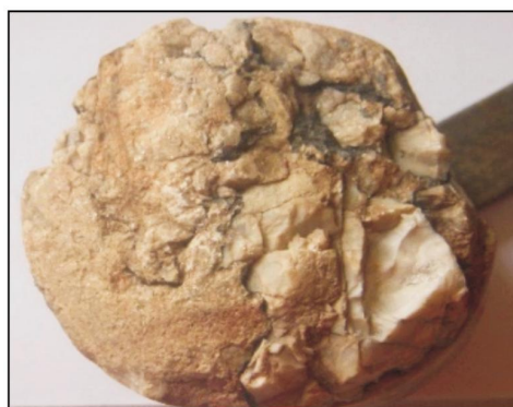
(c) 中晶白云岩,见硅质角砾岩。罗斯2井5745.65~5 745.81 m,蓬莱坝组。岩心
